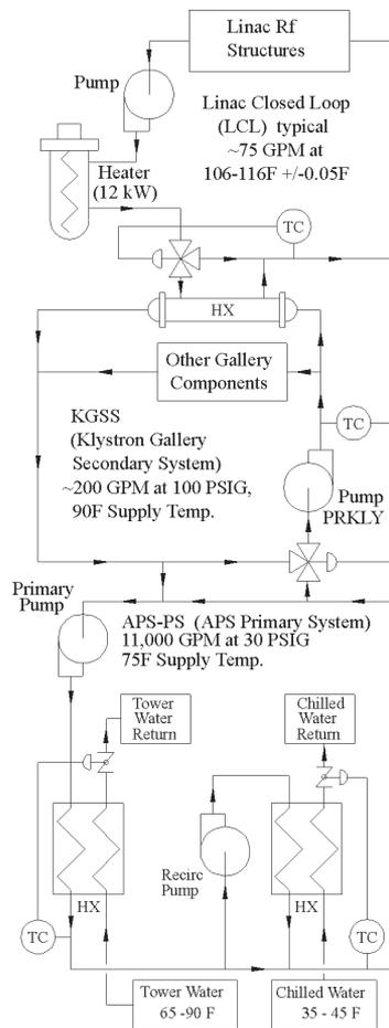
Figure 2: Overview of the linac water system.
