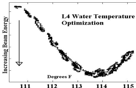
Figure 1: The optimal temperature for L4 is  $\approx 113.7$  °F.
