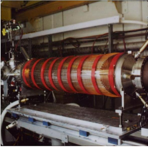
Figure 2: Photo of kicker on ETA-II beam line. White cables (unconnected in this picture) connect pulsed to kicker. Red tape holds bias dipole magnet windings to outer shell of kicker.
