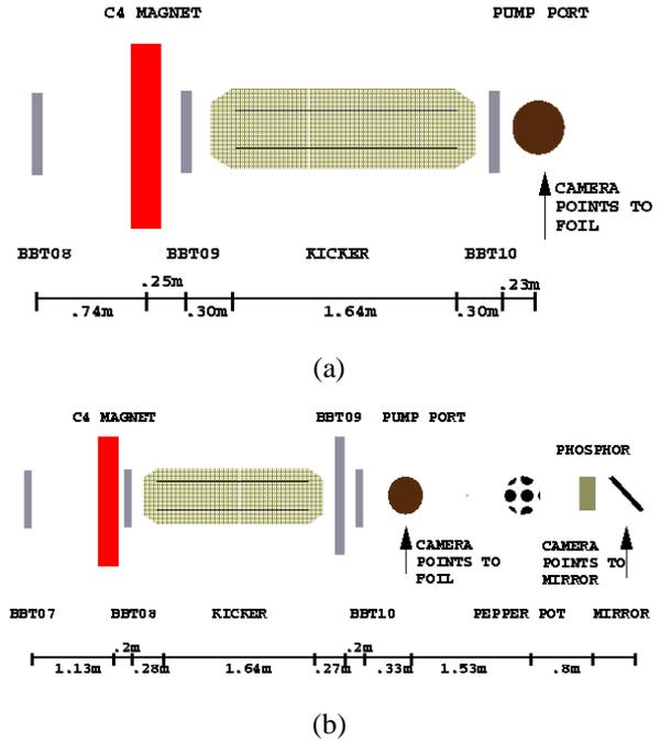
Figure 4: a) Old beam line layout. b) New beam line layout.
