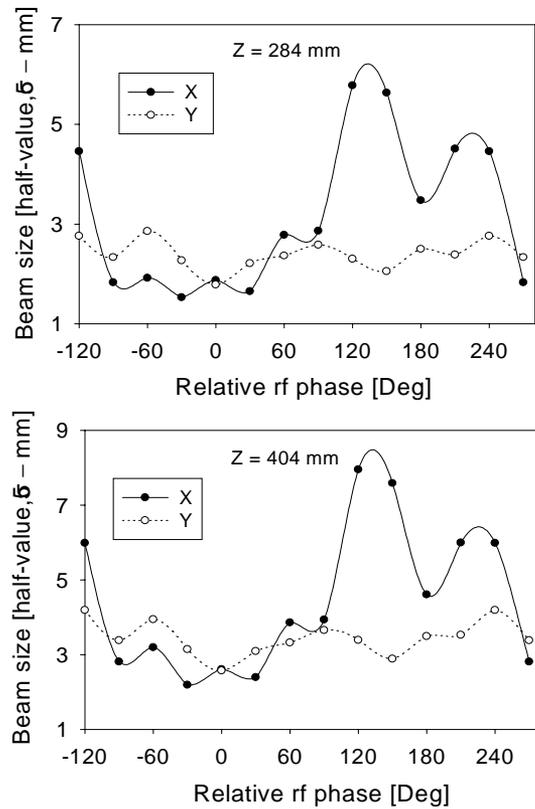
Figure 5. Calculated output beam dimensions at 284 mm (top) and 404 mm (bottom) from RFQ2 exit.
