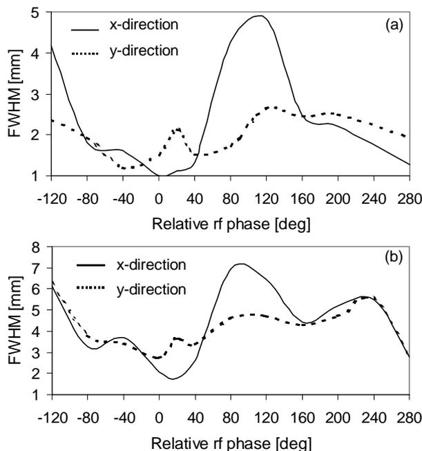
Figure 4. Measured beam dimensions at 284 mm (top) and 404 mm (bottom) distance from RFQ2 exit.
