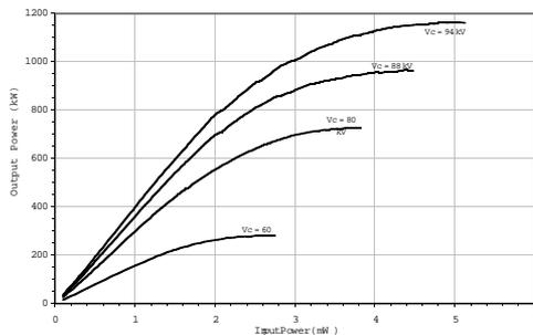
Figure 2. Output power characteristics.
