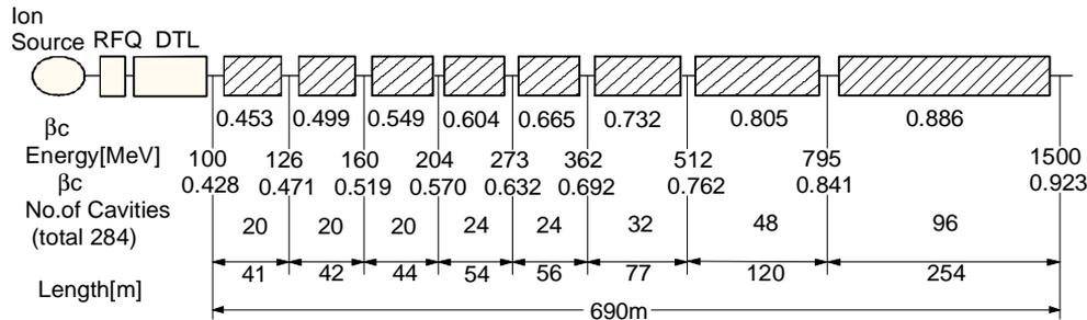
Fig. 6 Basic parameters for superconducting(SC) linac.
