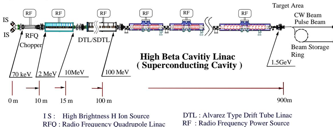
Fig. 1 A conceptual layout of the JAERI NSP-LINAC
