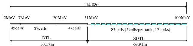
Fig. 5 A concept of DTL and SDTL
