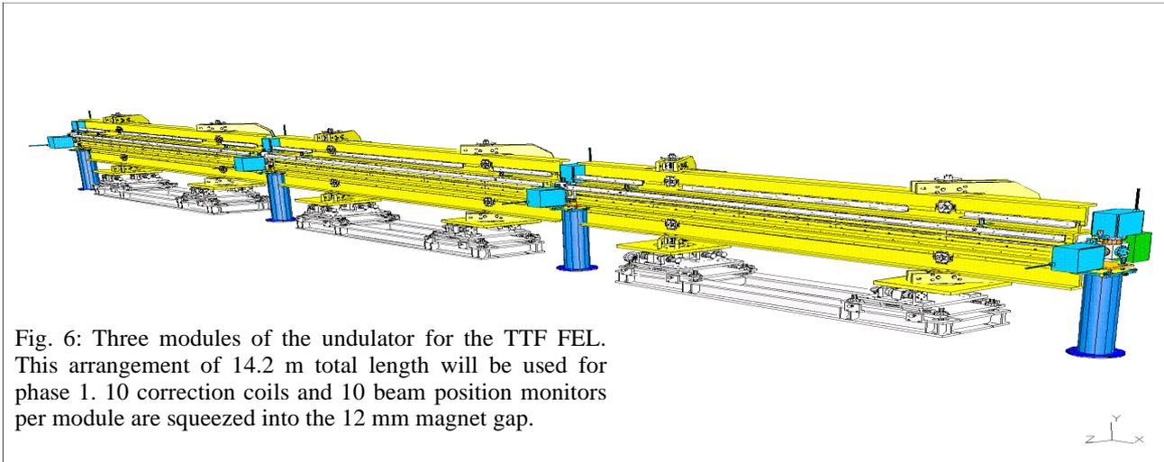
Fig. 6: Three modules of the undulator for the TTF FEL. This arrangement of 14.2 m total length will be used for phase 1. 10 correction coils and 10 beam position monitors per module are squeezed into the 12 mm magnet gap.
