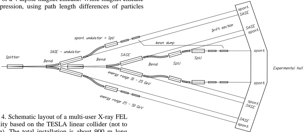
Fig. 4. Schematic layout of a multi-user X-ray FEL facility based on the TESLA linear collider (not to scale). The total installation is about 900 m long and 200 m wide and would be located on the same site as the linear collider interaction region.
