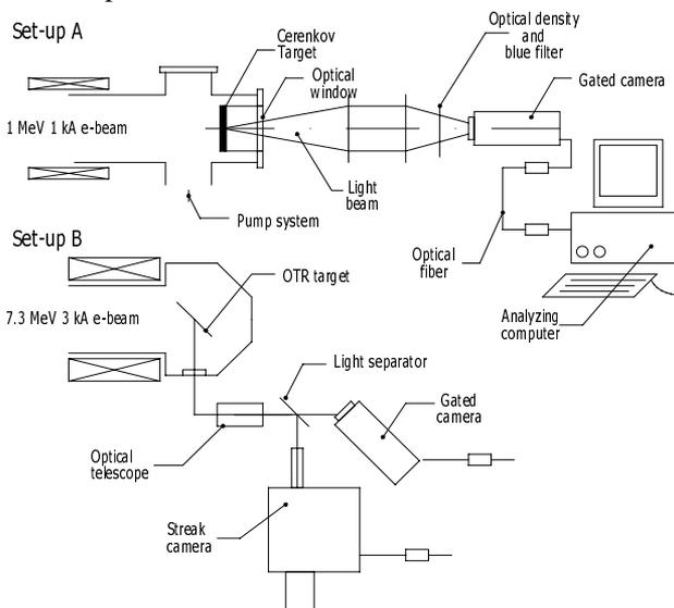
Figure 1: Schematic drawings of the two different set-up.
