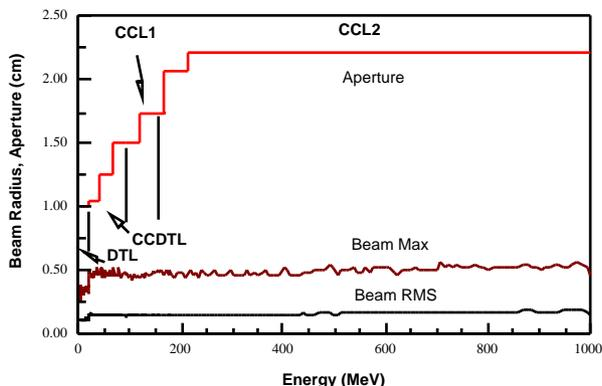
Figure 2. Aperture and beam size in the linac
