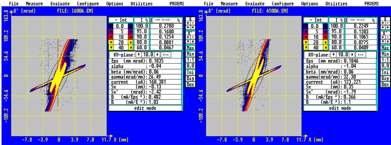
Figure 3: Comparison between the emittances of the extracted beams of the two ion sources at 0.8 mA. The ellipses correspond to the 90% normalized KV-emittances which are  $\epsilon_{KV} = 0.1835 \pi$  mm mrad for the first source and  $\epsilon_{KV} = 0.1846 \pi$  mm mrad for the second source.
