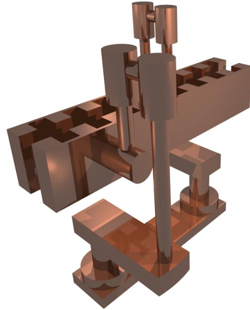
Figure 7: View of the multi-gap funneling deflector.
