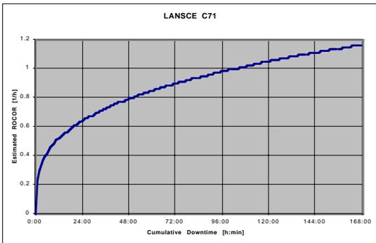
Figure 7. Estimated ROCOR - Rate of Occurrence of Repairs
