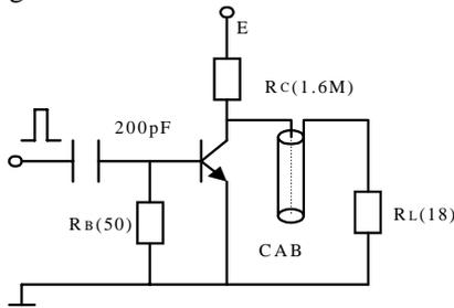
Figure 3. Circuit diagram of the ns pulser
