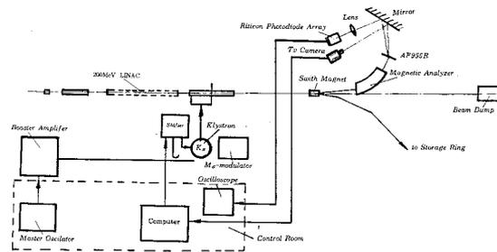
Figure 2. Layout of the automatic energy stabilizer
