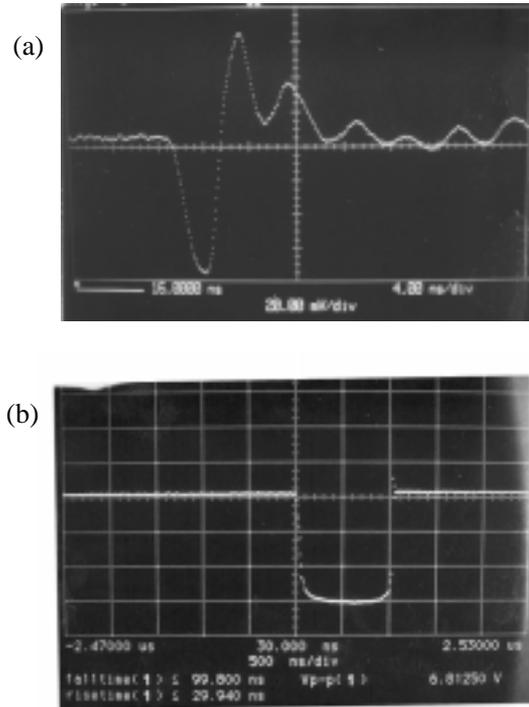
Figure 5. Waveform of output voltage of the combination pulser (a) ns waveform, (b)  $\mu\text{s}$  waveform
