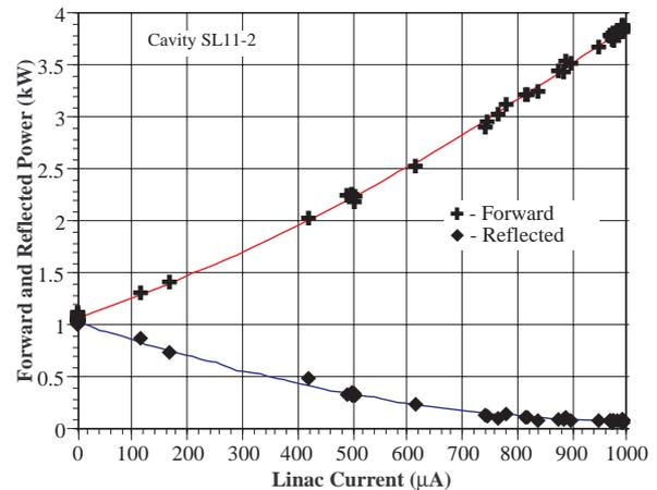
Figure 1. Matched rf load at full current.
