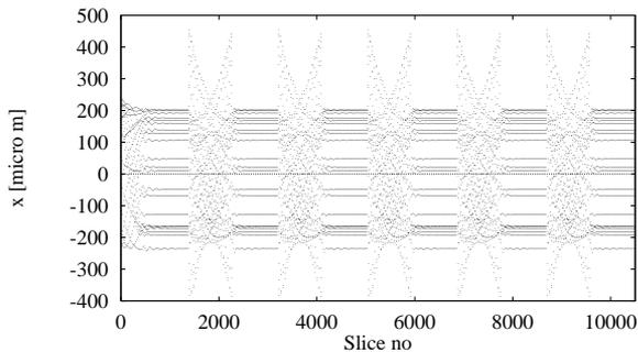
Figure 3: The final slice position for detuned structures with  $Q = 100$ . Each bunch is cut longitudinally into 21 slices, the first 500 bunches are plotted. The horizontal lines visible, are formed by equivalent slices of successive bunches. The slices of each bunch are filling the space between the minimum and maximum position.
