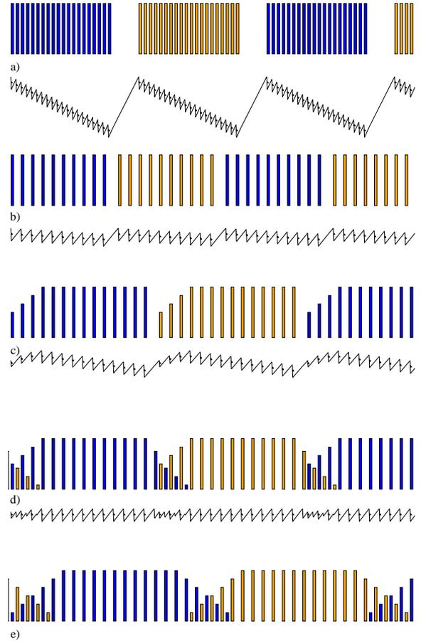
Figure 1: The charge distribution along the pulse—in case a) different trains are shown in different tones, in the other cases different half-trains are shown different tones. The number of bunches on the flat top is constant but different from the real value. The curves indicate the variation of the energy gain. Depending on the injector, a distribution in the range of d) to e) will be chosen.
