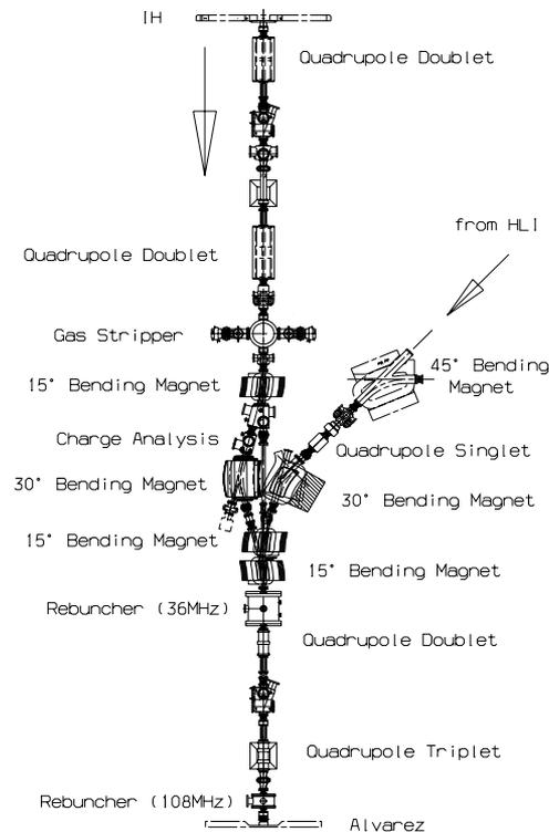
Figure 2: Layout of the new stripper section.
