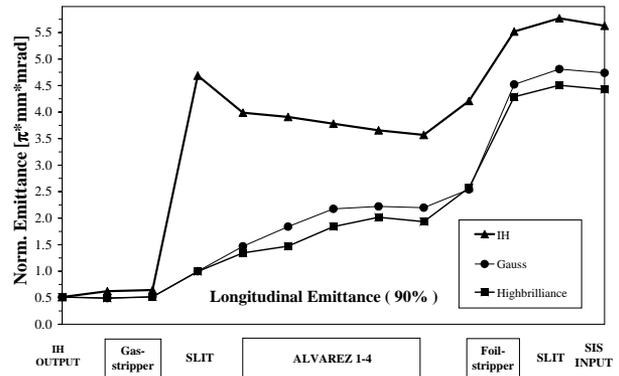
Figure 4: The longitudinal 90% emittances complementary to Fig. 3.
