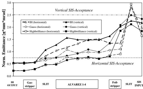
Figure 3: Variation of the horizontal and vertical 90% emittances from the UNILAC stripper section to the SIS input for different input beams. The transmission in all cases is approx. 95%.
