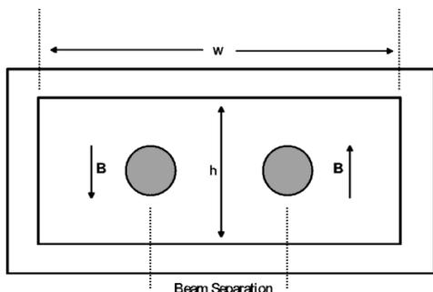
Figure 4 Magnetic dipole septum magnet
