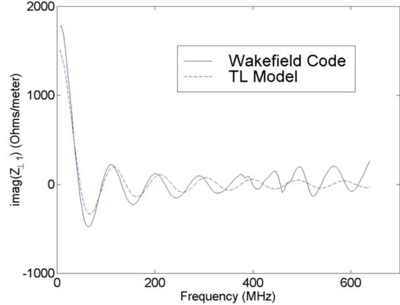
Figure 2 Dipole wake impedance
