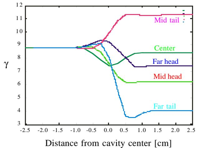
Figure 2. Fiducial trajectories in an rf cavity
