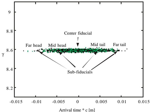
Figure 1. Initial fiducial coordinates and beam distribution in longitudinal phase space.
