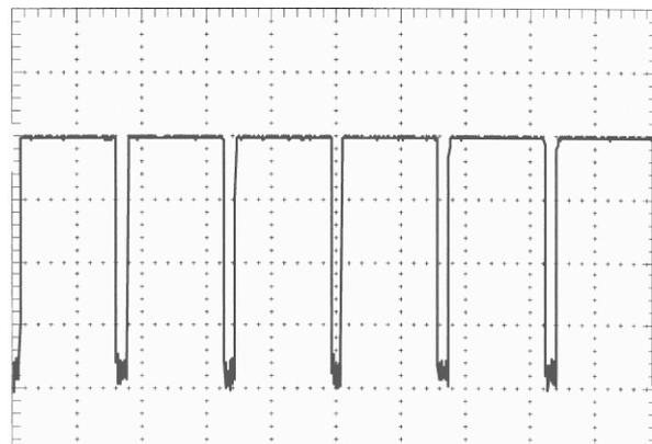
Figure 6: An oscilloscope display of the H<sup>-</sup> pulse at 12% duty factor. The vertical scale is 10 mA/div. The time scale is 5 msec/div.
