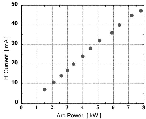
Figure 4: Plot of H<sup>-</sup> current as a function of arc power
