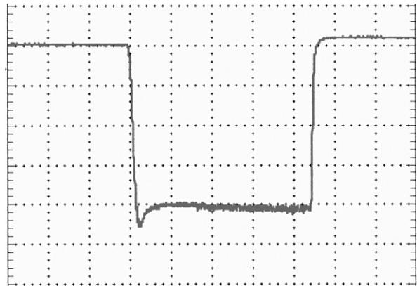
Figure 5: An oscilloscope display of the 40 mA H<sup>-</sup> pulse. The vertical scale is 10 mA/div. The time scale is 250 μsec/div.
