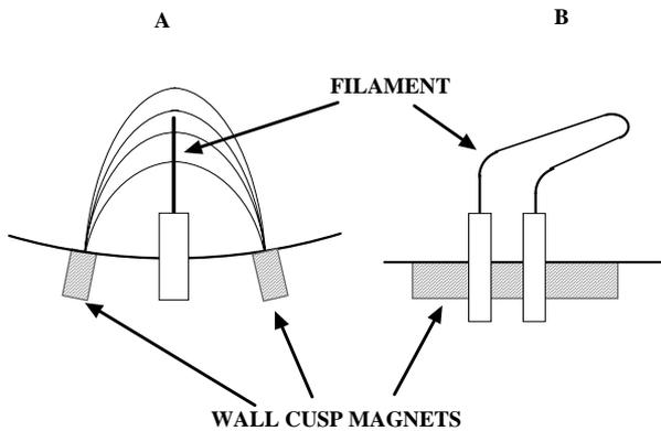
Figure 3: Location of the filament within the wall cusp magnet field. A. View along longitudinal axis. B. Viewed side on.
