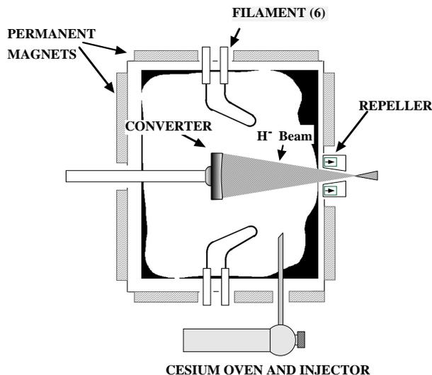
Figure 1: Schematic of the surface conversion ion source.
