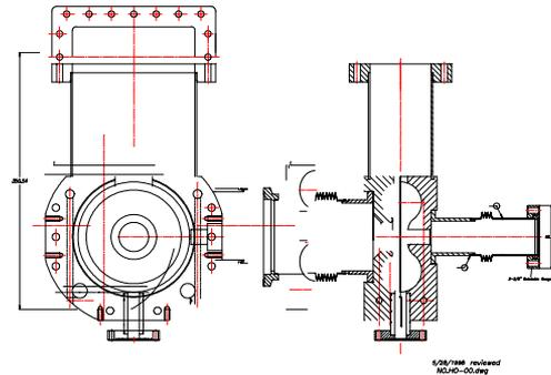
Figure 1: Assembly drawing of the gun cavity
