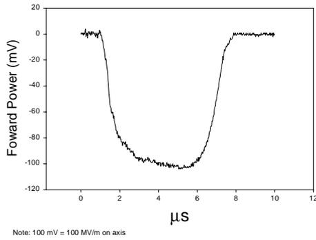
Figure 6: Measured forward rf power to the gun. This is a scope trace that measures envelope of rf pulse with calibrated diode detector. The peak voltage corresponds to 2 MW peak rf power.
