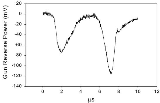
Figure 7: Reflected rf power from the gun. It shows that after the gun was filled, no reflection was observed.
