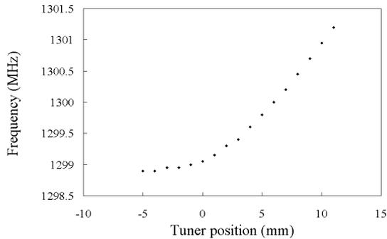
Figure 3: Measured resonant frequency dependence of tuner position.
