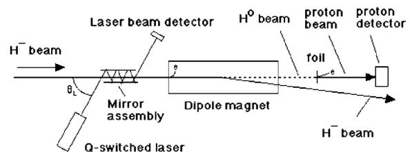
Figure 3. A generic arrangement for laser beam diagnostics.
