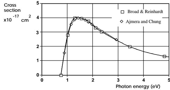
Figure 1. Photodetachment cross section of H<sup>-</sup> vs. photon energy in the H<sup>-</sup> rest frame.
