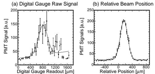
Figure 2: Result of a position jitter subtraction to magniscalle readout position of wire scanner. (a) PMT signals as a function of wire readout position, (b) PMT signals as a function of evaluated relative beam position to wire.
