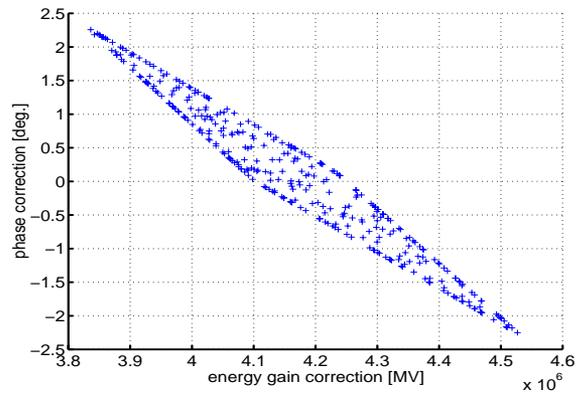
Figure 4: Energy gain and beam phase correction range at the low energy end of Linac 1. The vector sum of 2 cavities is controlled and varied by  $\pm 3$  deg. in phase and  $\pm 10\%$  in amplitude.
