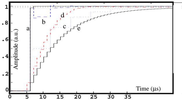
Figure 3: Step response of the transfer Function  $G_{Ty}$  for a) optimal SP b) SP with 20% lower cavity quality factor c) SP with 50% gain decrease due to klystron nonlinearity d) normal feedback with gain of 70 e) SP with gain of 70.
