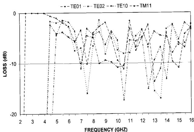
Figure 6. Propagation loss of first four waveguide modes in the waveguide harmonic damper.
