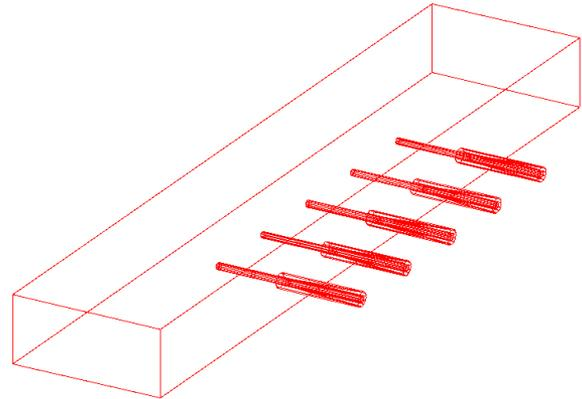
Figure 3. Damper structure with coaxial probe antennas.
