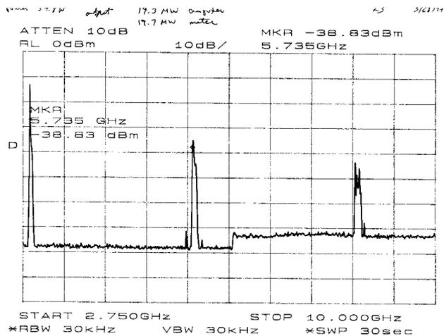
Figure 1. Harmonic spectrum of 2.856-GHz klystron amplifier output.
