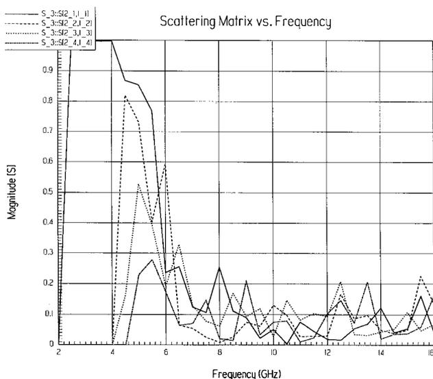
Figure 5. Transfer characteristics of waveguide modes through the harmonic damper.
