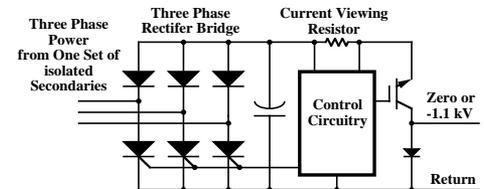
Figure 2: Each module contains independent control circuitry to disable the module in the event of module control failure.
