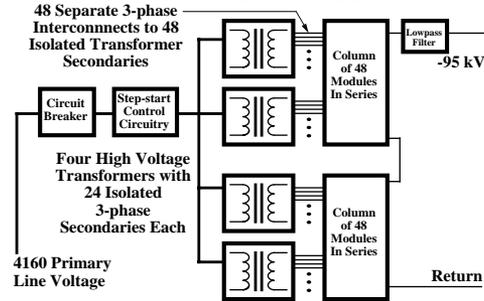
Figure 1: Two transformers serve each power column.
