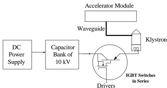
Fig 4. Block diagram of the series high voltage modulator.
