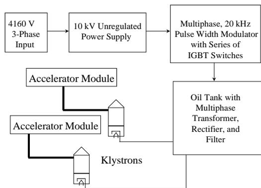
Fig. 2. Block diagram of the fast converter modulator.
