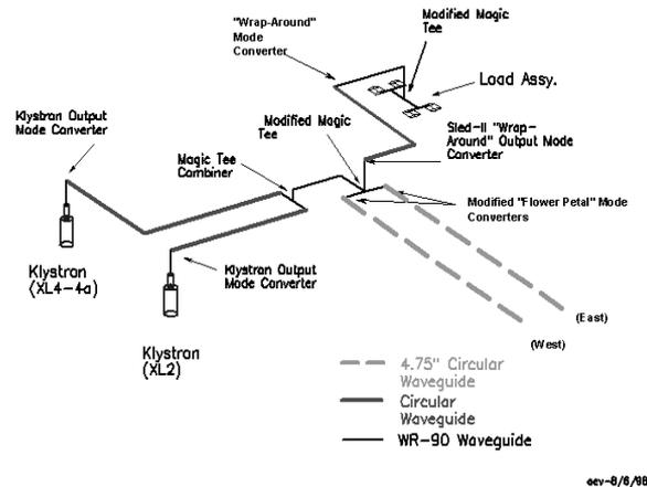
Figure 1. Schematic of the initial experimental setup.
