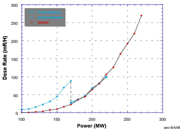
Figure 2. Radiation Intensity at the SLED-II Magic Tee.
