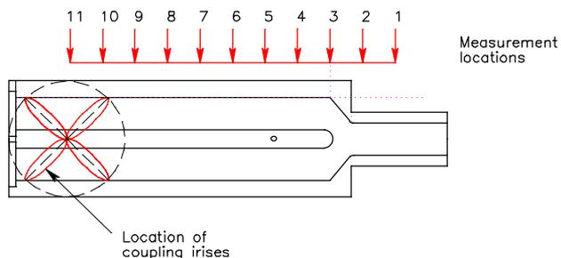
Figure 4. Location of measurement points along the rectangular portion of the mode converter. Additional measurement points are located out of the paper along the circular portion of the converter.
