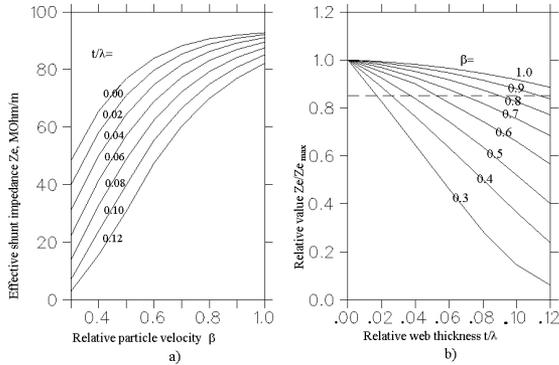
Figure 3: Effective shunt impedance  $Z_e$  for different web thickness a) and reduction in  $Z_e$  with increasing of the web thickness b).
