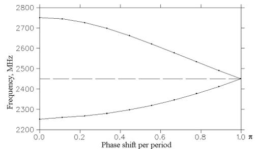
Figure 4: Dispersion curves for operating passband (experiment).
