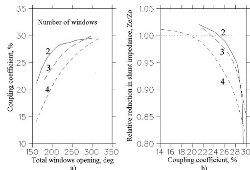
Figure 2: Parameters of the CDS structure
