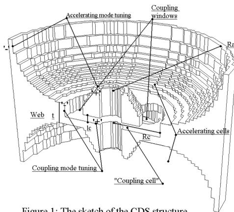
Figure 1: The sketch of the CDS structure.
