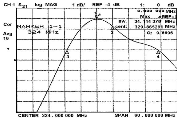
Fig.5 Spectrum of  $S_{21}$  showing the  $Q_L=9.7$ .
