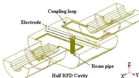
Fig.1 RF deflector cavity with large coupling loops.
