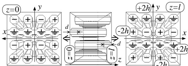
Figure 7: MB-RFQ resonator with 4x4-matrix array of electrodes.
