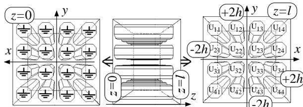
Figure 3: MB-RFQ resonator with a 4x4-matrix array of electrodes allowing an observation of normal modes.
