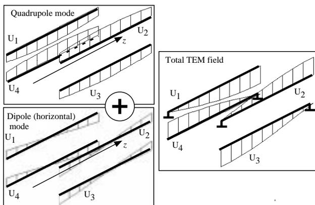
Figure 8: The superposition of quadrupole and dipole modes shifted by  $\lambda/4$  to each other.
