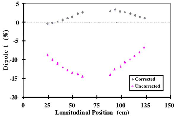
Figure 2. Dipole 1 contribution to the quadrupole field distribution.
