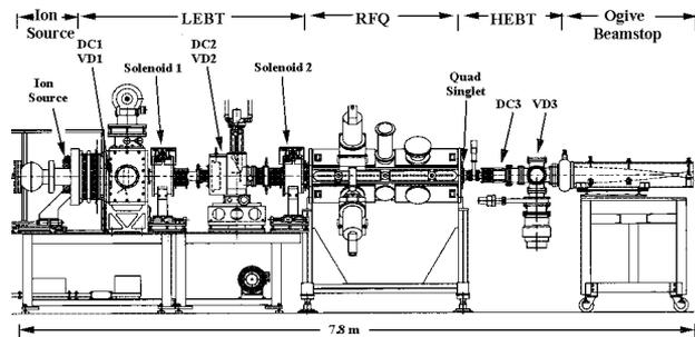
Figure 1. The LEDA Injector/CRITS RFQ experiment beamline.
