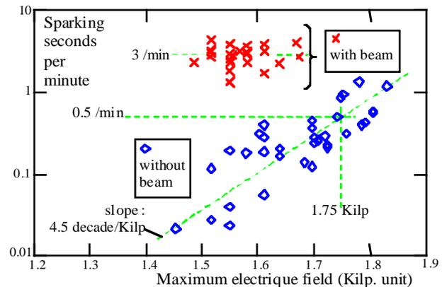
Figure 5. Average spark rates during long runs.
