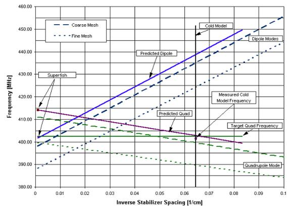
Figure 1 – Computer analyses of the quadrupole and dipole modes as a function of stabilizer spacing.
