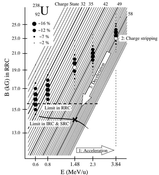
Figure 1: Principle of the CSM. The size of the dots corresponds to the production rate of Uranium ions with respective charge state at the stripping energy,  $E$ , when using a carbon foil for the stripper. The ordinate represents the necessary bending power in the RRC. The bending limit in the IRC and SRC is also indicated.
