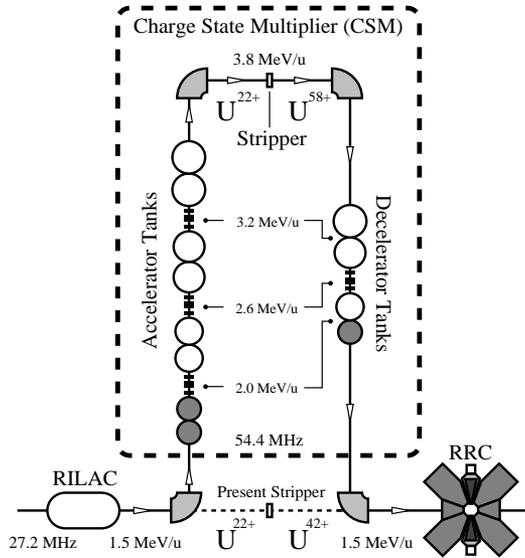
Figure 2: Schematic layout of the CSM. The energies at the fundamental frequency of 27.2 MHz are also indicated.
