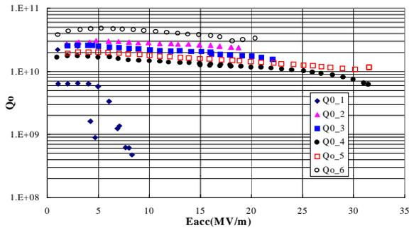
Figure 1:  $Q_o$  vs.  $E_{acc}$  at SHI-1 cavity.
