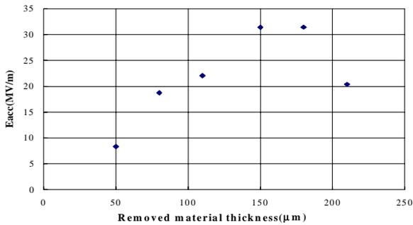
Figure 2:  $E_{acc}$  vs. removed thickness on SHI-1 cavity.
