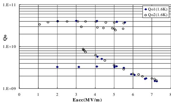
Figure 5:  $Q_0$  vs.  $E_{acc}$  at SHI-3 cavity.
