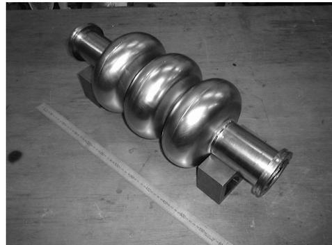
Figure 7: Overall view of 3 cell-cavity.
