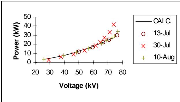
Figure 4. Voltage versus Power for the RFQ
