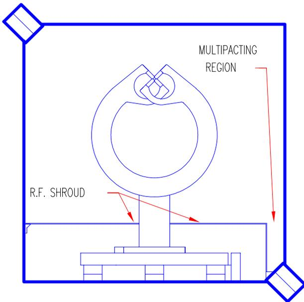
Figure 5. Cross-section schematic of RFQ tank and rings
