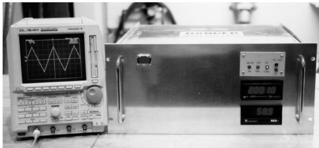
Figure 6: Modulator and test waveform (+/-100 A, 500 Hz)
