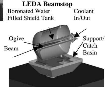
Fig. 6 Beamstops built and operated for ED&D
