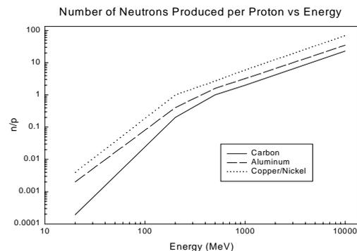
Fig. 1 Comparison of beam absorber materials
