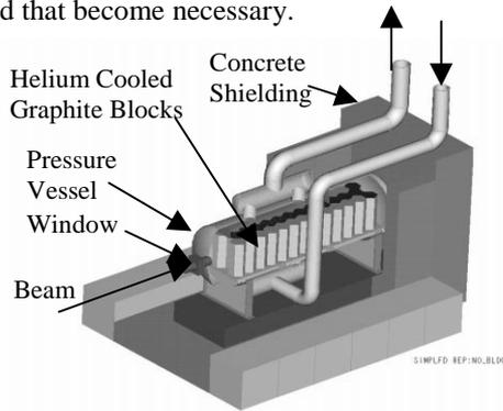
Fig. 5 High energy beamstop – 1700 MeV
