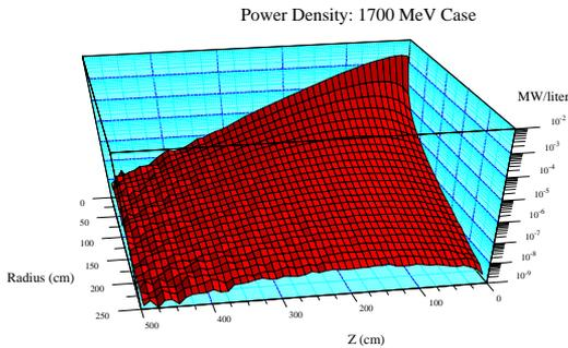
Fig. 3 Power density in graphite from a 1  $\sigma = 2.66$  cm 1700 MeV proton beam
