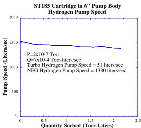
Figure 5. Measured Speed of ST185 Cartridge Pump.
