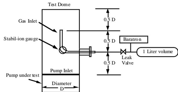
Figure 1. Test setup for pump speed measurement.
