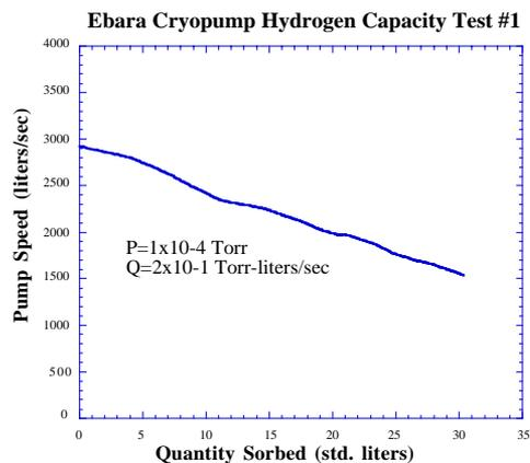
Figure 3. Measured Cryopump Capacity at High Flow.
