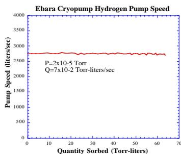
Figure 2. Measured Cryopump Pump Speed Versus Sorption.
