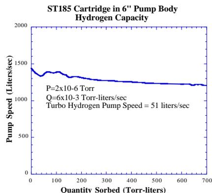
Figure 6. Measured Capacity of ST185 Cartridge Pump.
