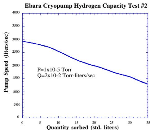
Figure 4. Measured Capacity at the Lower Flow Rate.
