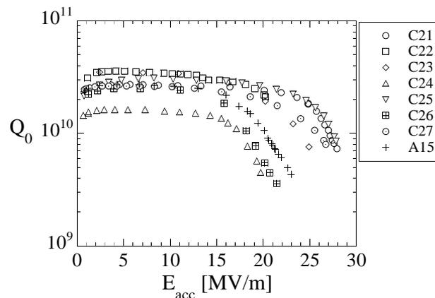
Fig. 3: Vertical test results of the 8 cavities selected for module 2.
