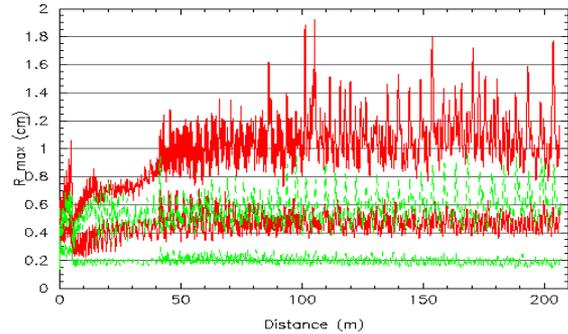
Figure 1. Evolution of the maximal beam radius along the linac with errors (upper lines) and without errors (i.e. design linac) with space charge (solid lines) and without space charge (dashed lines).
