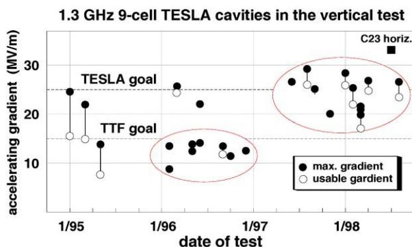
Fig. 1: Vertical test of 1.3 GHz 9-cell cavities.
