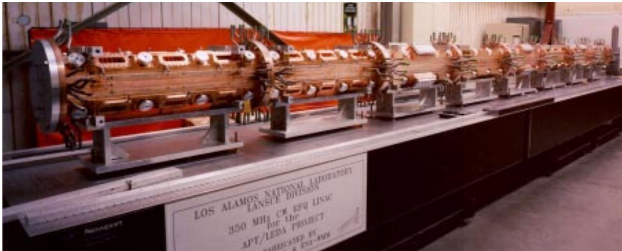
Figure 4: APT/LEDA RFQ Assembled for Pre-Installation RF Tuning
