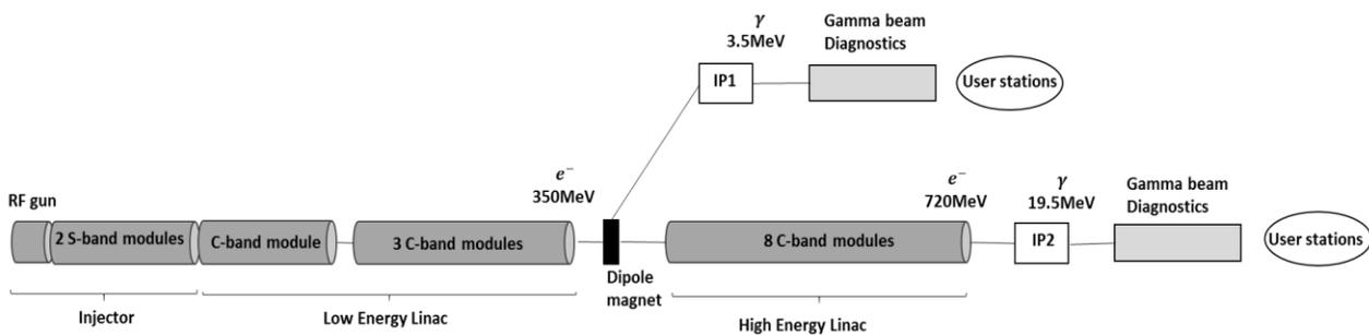
Figure 2: Schematic layout of the Gamma Beam System.
