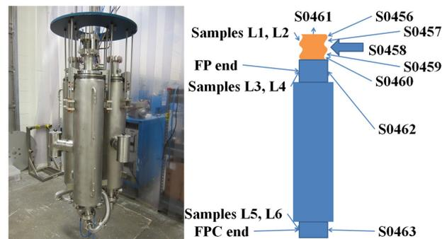
Figure 1: Bellows attached cavity on a test stand waiting to be loaded into the Dewar (left). Sampling locations on CAV0278-Bellows 2068 (right).
