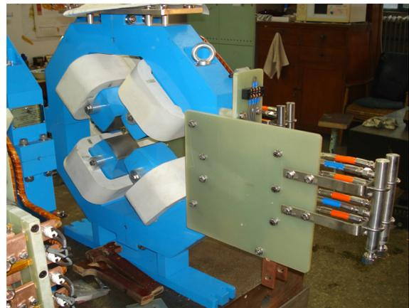
Figure 3: NSC KIP 100 MeV/100 kW linear accelerator quadrupole lens.
