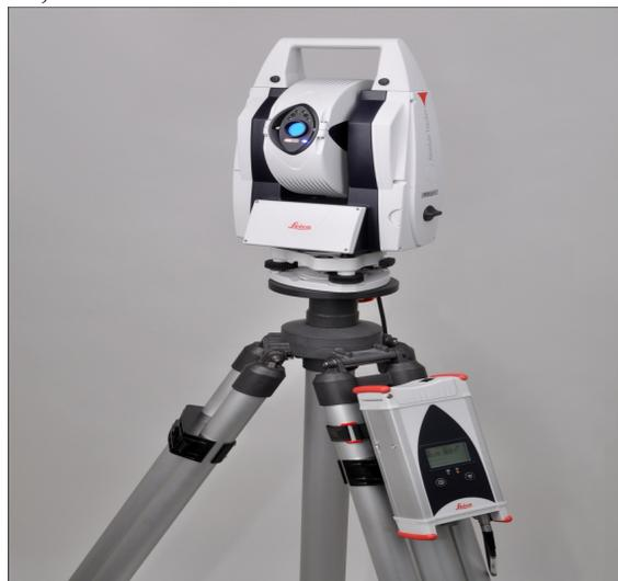
Figure 1: The Leica Absolute Tracker AT401.
