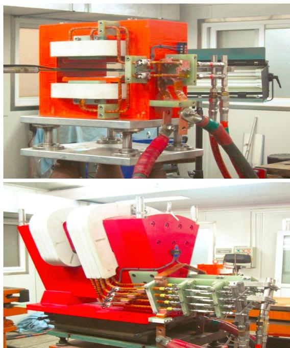
Figure 4: NSC KIPT 100 MeV/100 kW linear accelerator first chicane magnet, 45 degree bending magnet.
