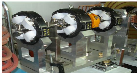
Figure 5: NSC KIPT 100 MeV/100 kW linear accelerator quadrupole triplet.
