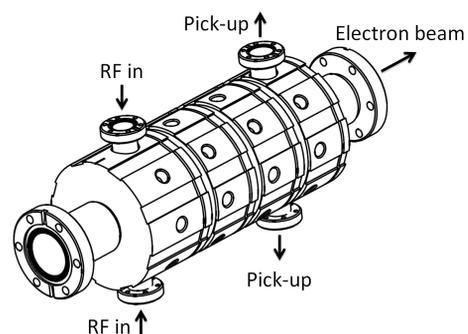
Figure 1: Technical design of the 4-cell fast corrector cavity with the 2 beamline flanges and the 4 feedthroughs for RF input and output loops/pickup.
