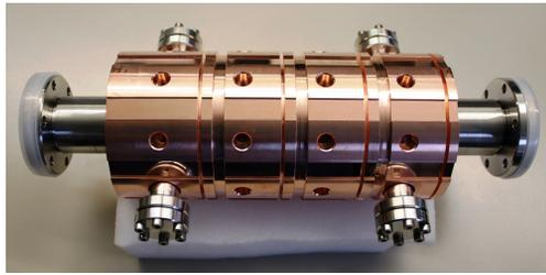
Figure 2: Assembled cavity after cell production, complete soldering and initial cleaning. The input and output loops are not connected.
