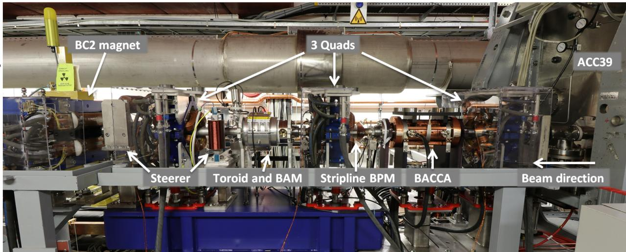
Figure 3: Picture from the installation during shutdown in January 2018. Beam direction is from right to left, with third harmonic RF module (ACC39) to the right and the entrance of the first bunch compressor (BC2) to the left.
