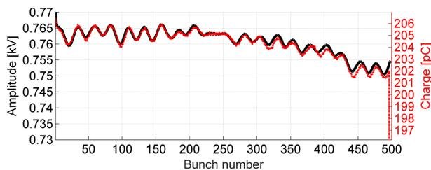
Figure 4: Maximum bunch transient amplitude in comparison to the charge measurement in the BC2 section. The black curve shows the maximum peak voltage and the red dashed line the charge readout for each bunch.
