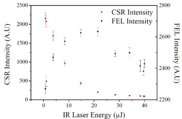
Figure 6: CSR intensity and FEL intensity as a function of IR laser heater energy.
