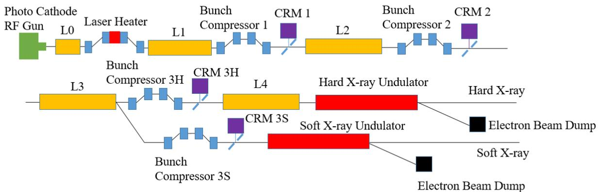
Figure 1: Schematic structure of PAL X-FEL.
