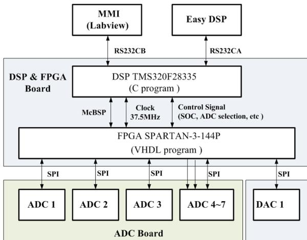
Figure 3: Interface signals between devices in the MPS.
