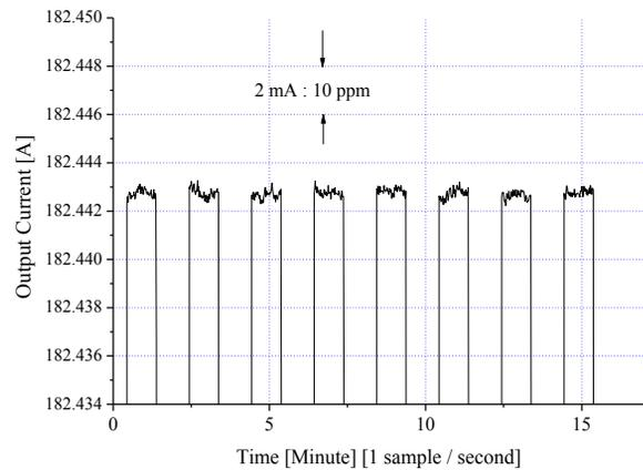
Figure 9: Repeatability test results. This shows about 4 ppm-pp.
