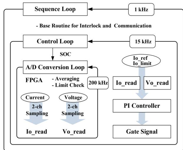
Figure 4: DSP and FPGA program timing assignment.
