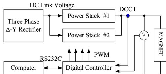
Figure 1: The block diagram of the developed MPS.
