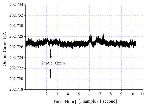
Figure 7: Long term output current stability.
