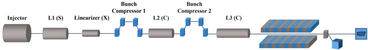
Figure 1: Layout of the SXFEL user facility linac including the injector section, S-band sections (L1), one X-band linearizer (LX), C-band sections (L2, L3) and two bunch compressor chicanes (BC1, BC2).
