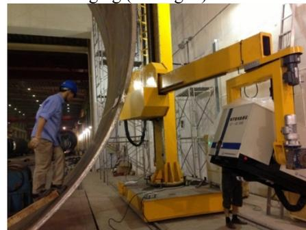
Figure 2: NDT accelerator on duty.
