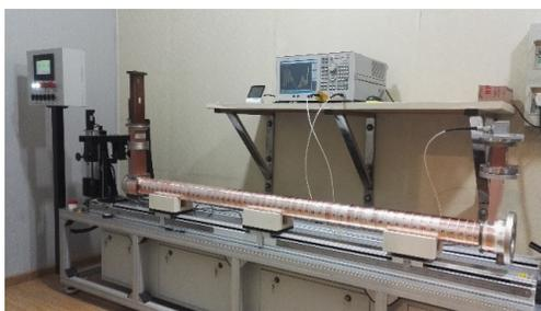
Figure 5: Travelling wave accelerating tube tuning.
