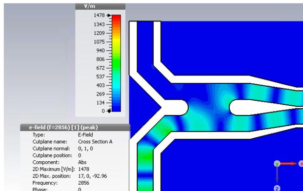
Figure 4: Distribution of the electric field component in the cross section of the 3-dB coupler.
