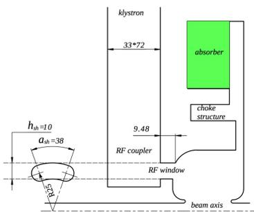
Figure 3: Arrangement of RF energy input.
