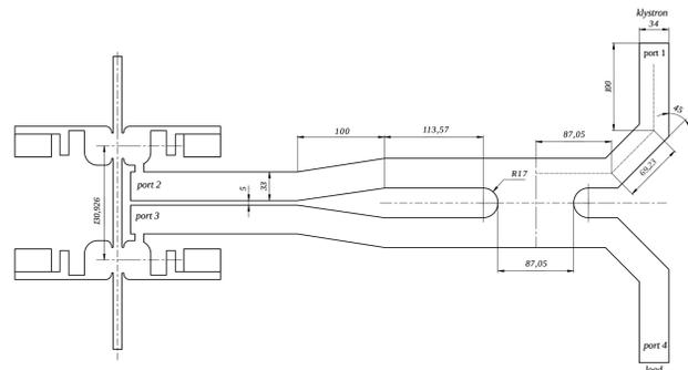
Figure 2: The design of the two cavities resonator fed through a 3-dB coupler.
