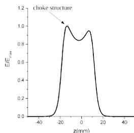
Figure 5: Distribution of the electric field of the operating mode along the axis of the cavity.
