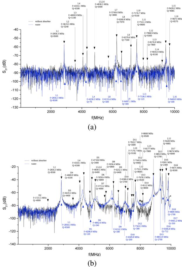
Figure 7: Measured spectra of (a) longitudinal modes, (b) dipole modes. Black curve — measurements without an absorber, blue curve — with an absorber.
