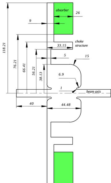
Figure 1: Geometry of the RF resonator.
